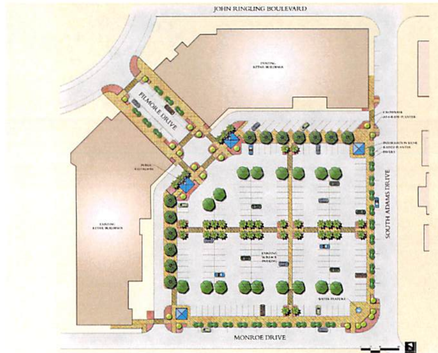
Figure 3-23: Surface Parking Improvement Concept Plan, South (Aqua) Quadrant. Improvements above will result in a net loss of forty-three (43) spaces, but is recommended to improve the function of the lots and the image of St. Armands. This concept has been provided in the case that the G zoned lots will not be developed within a short time frame.
