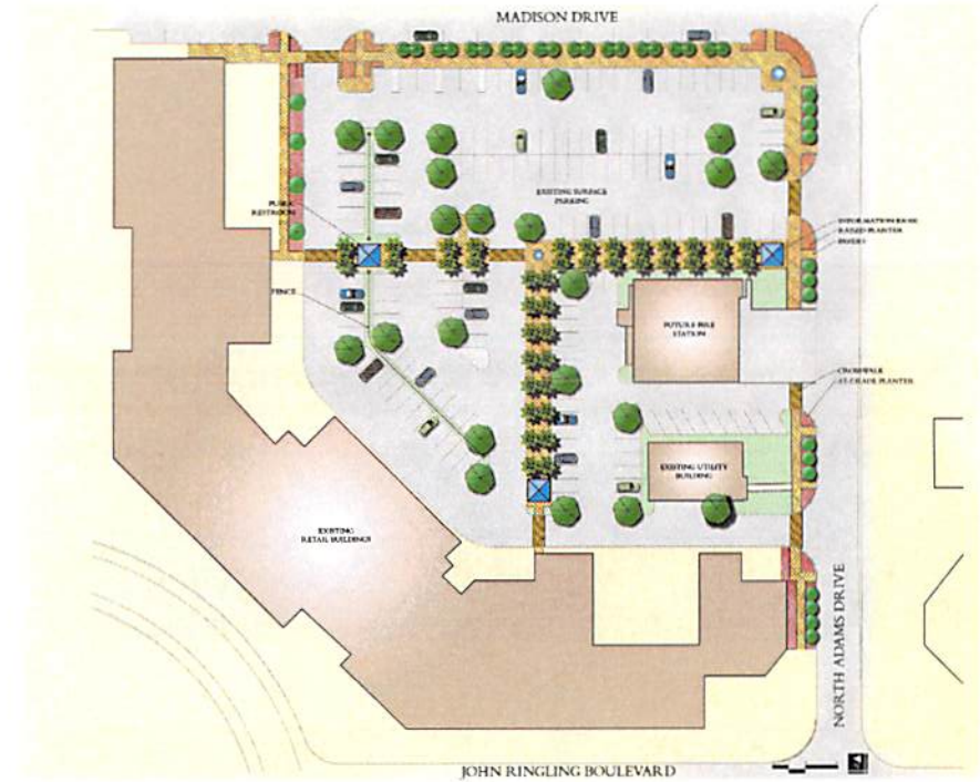
Figure 3-24: Surface Parking Improvement Concept Plan, North (Gold) Quadrant. Improvements above will result in a net loss of twenty-five (25) spaces, but is recommended to improve the function of the lots and the image of St. Armands. This concept has been provided in the case that the G zoned lots will not be developed within a short time frame.
